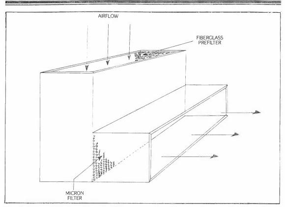
Figure 239 A standard design of a laminar flow cabinet for tissue culturists.
