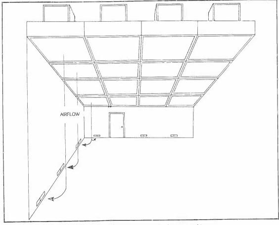
Sterile room with ceiling composed of micron filters. Figure 241
