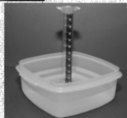
Reading the amount of oxygen in the graduated cylinder.
